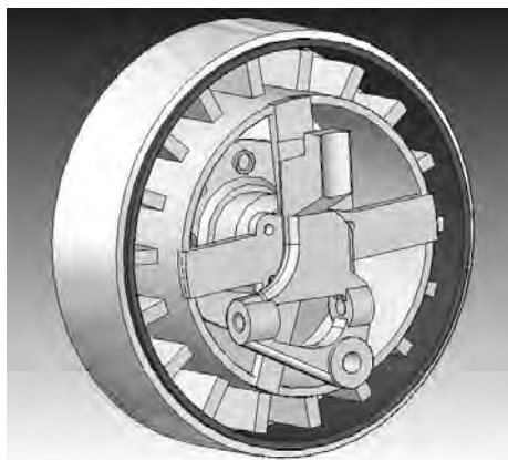
Rys. 5. Stator i rotor silnika Fig. 5. Engine stator and rotor
